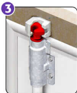
3 Cam rotating over center.
