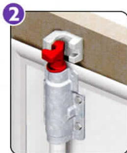
2 Cam leveraging door towards closed position.
